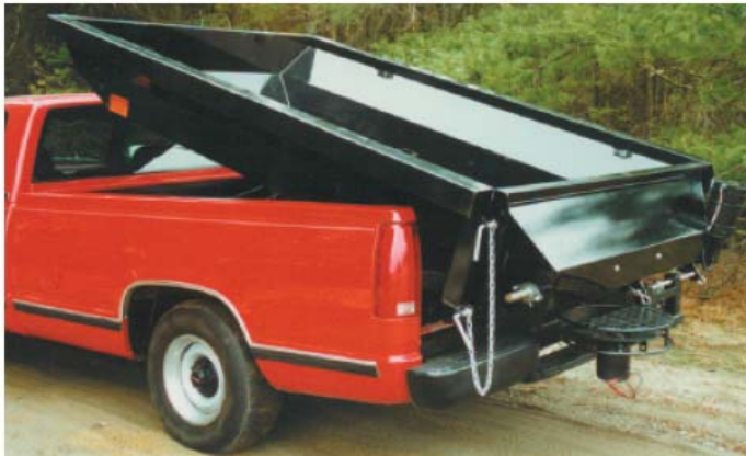
The Junior — has a 4' hopper, can be used on a utility vehicle or in a pickup. Choose from 1/3 or 2/3 yard capacity.
