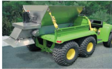
The Junior — has a 4' hopper, can be used on a utility vehicle or in a pickup. Choose from 1/3 or 2/3 yard capacity.
